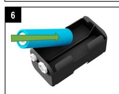
Fit the 4 batteries into the holder.
