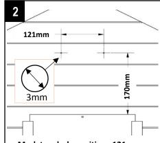
Mark two hole positions 121mm apart and approximately 170mm above the top of the sliding door.
