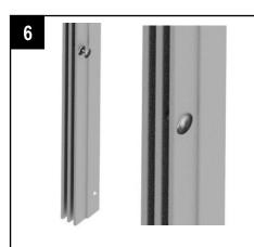
Locate the rivet in the hole, then push it in to secure it.
