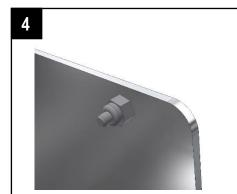
Tighten each nut by turning the screw with a screwdriver whilst holding the nut with pliers or a spanner.
