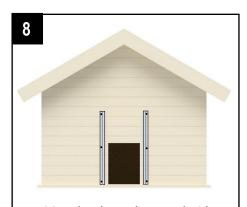
Position the channels on each side of the door hole on the hen house with the hole central between the channels. They must be perfectly vertical, flat and level. The fixing holes must be 322mm – 325mm apart.
