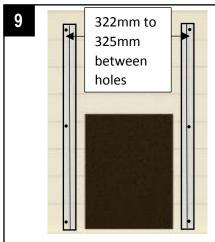
Once the channels are vertical and the holes are 322mm – 325mm apart, mark the locations for the six fixings. Drill 1.5mm diameter holes.
