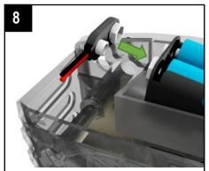
Fit the connector to the battery holder.
