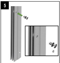
Fit a plastic rivet (d) to each channel in the hole shown.
