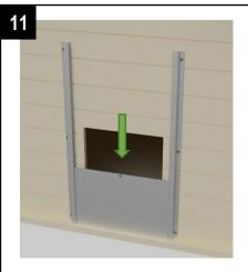
Slide the door panel with grommet down the channels.
