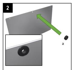
Fit the grommet (a) to the centre hole in one door panel.
