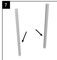
The channels are fitted to the hen house with the rivets at the bottom of each channel, not nearer to the top.
