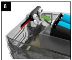
Fit the connector to the battery
