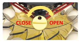
Opening and closing the vent: Close the vent to increase humidity or open the vent to decrease humidity.
